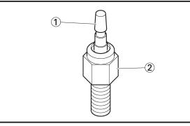
Measure the carburetor heater resistance.
