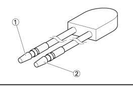
Check the thermo switch for continuity at the temperatures indicated below.
